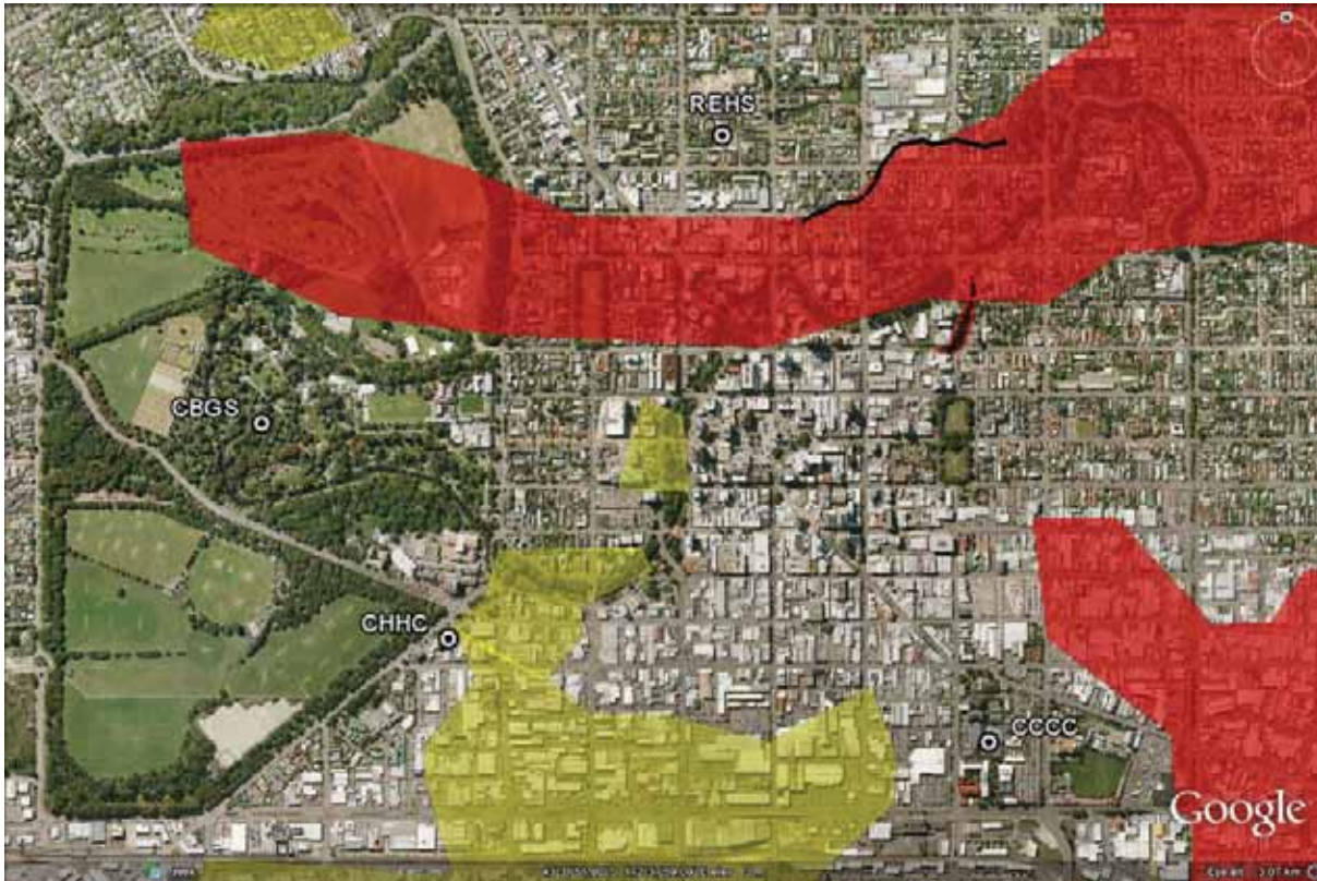
Figure 2: Preliminary liquefaction map indicating areas within the CBD affected by liquefaction in the 22 February earthquake. Red = moderate to severe liquefaction; green = low to moderate liquefaction (source: Cubrinovski and McCahon, August 2011)
