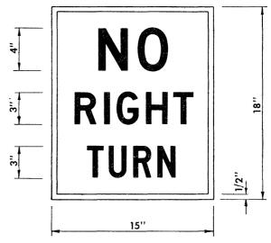
The sign shall consist of a black rectangle surrounded by a red border of translucent material and bearing the words "No Right Turn" in letters of white translucent material, and the sign shall be illuminated at all times by means of internal lighting.
